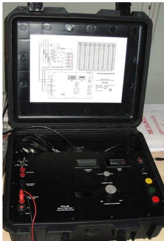
Picture 4: Photo of auxiliary device (over-current simulator)
