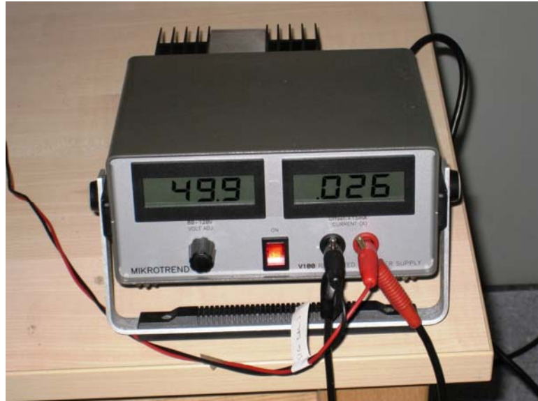
Picture 3: Photo of auxiliary device (DC power supply)
